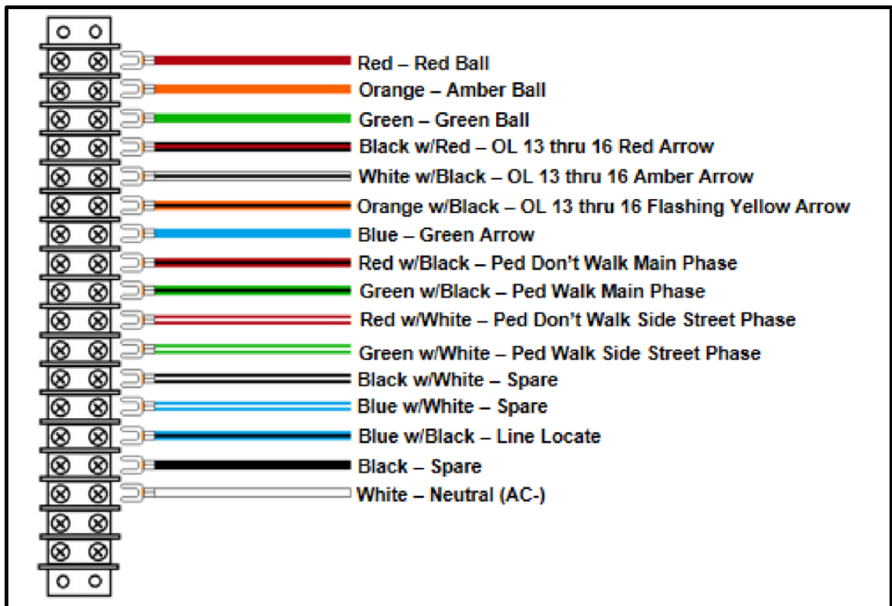
Figure 7.1: Terminal Block Layout for 16-Conductor Signal Cable
